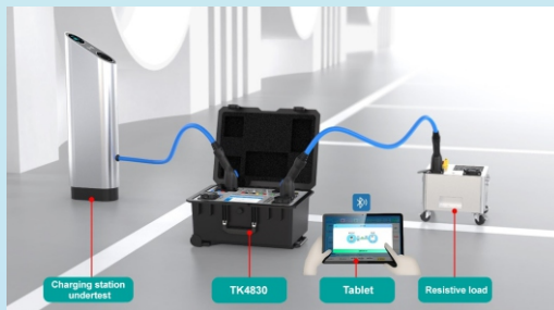
Test with resistive load as load
